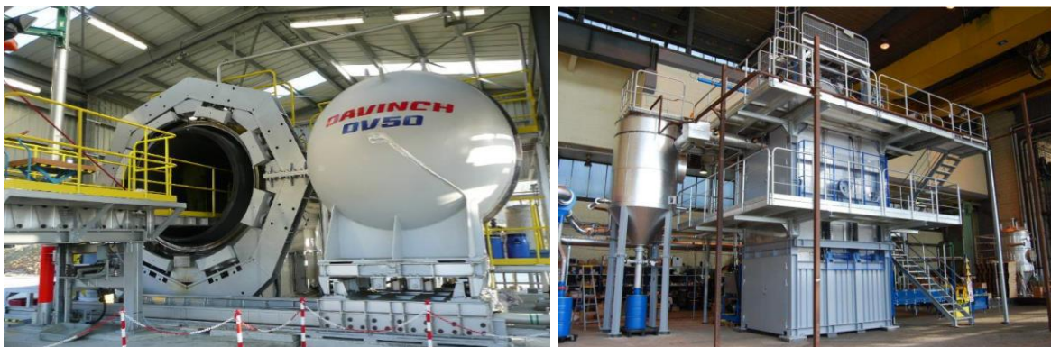
Left: The picture shows the heart of the system, the DAVINCH ® (Detonation of Ammunition in a Vacuum Integrated Chamber) vacuum furnace; Right: The SDC 1500 der Dynasafe based in Stockholm – Schweden
